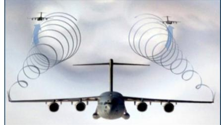
**Automated trail, at a safe distance, maintains position in wingtip vortex updraft.**
